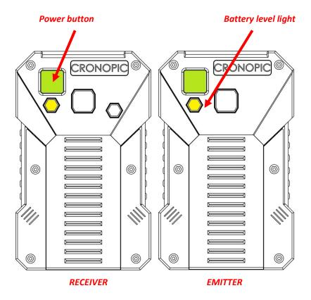
The blinking speed indicates the battery level as explained later.
